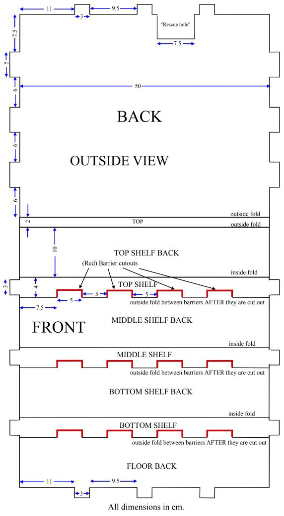
Apart from "rescue hole", design is left-right symmetrical. Tabs are either 3 or 5 cm width and 2 cm depth. Shelves are all the same dimensions.
